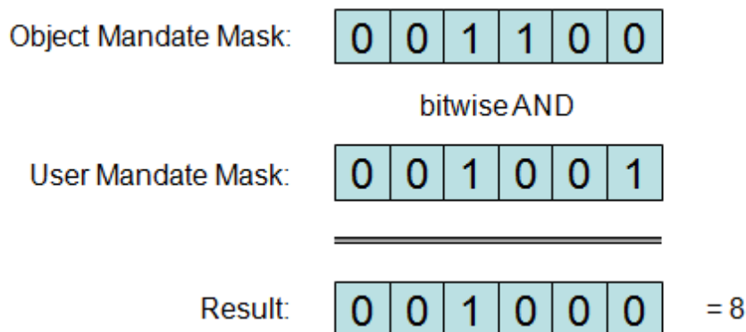
FIGURE: Calculation of the permission to an object based on the mandate masks of the current user mandate and the object
